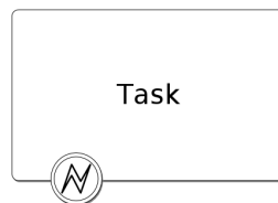
Figure 3.11: A task activity with attached error handler
